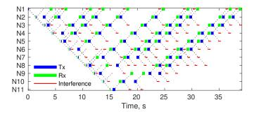
Fig. 5. LTDA-MAC schedule derived by the GA+PSO algorithm for the linear UASN deployed on a 20 km long pipeline.
