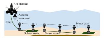
Fig. 1. Example of a linear UASN deployment for subsea asset monitoring.
